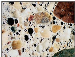
All concrete exposed to freeze-thaw action must be air entrained using chemical admixtures. Proper air entrainment involves the placement of very tiny air bubbles ( $\leq 1$  mm in diameter) within the concrete at a very tight spacing. These bubbles act to reduce the stresses created within the concrete when water expands during its transformation to ice during cold weather.
